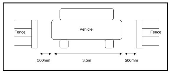
Figure 1: A schematic representation of the minimum dimensions applicable to servitude gates
