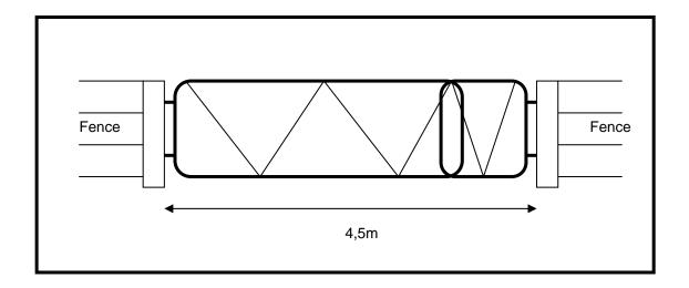
Figure 2: A schematic showing the use of two standard "Co-op" gates to cover the 4,5m gap.
